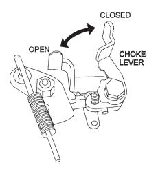
Figure 10. Choke Lever (Closed)
